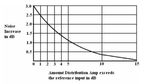
The DistAmp must ideally exceed the reference sources phase noise by at least 10 dB. Referring to the above graph, 10 dB (on the X axis) corresponds to 0.4 on the Y axis.
